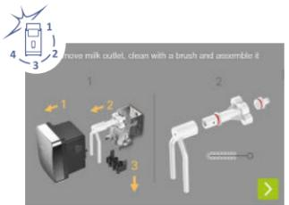
Remove the parts as shown on the display, clean them according to the hygiene concept and reassemble them. Follow the detailed instructions "Removal of the milk frother / coffee outlet" on the back page.
