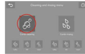
Press the COMBI-CLEANING button to start cleaning.
