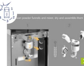
Remove the parts as shown on the display, clean them according to the hygiene concept and reassemble them. Follow the detailed instructions in the "Removal of the instant mixing unit" on the back page.
