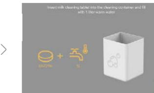
Fill the cleaning container with 1 litre of warm water and completely dissolve a milk cleaning tablet in it. Then hang the milk aspirator into the cleaning container. Also clean the milk container according to the hygiene concept.
