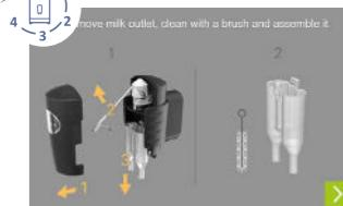
Remove the parts as shown on the display, clean them according to the hygiene concept and reassemble them. Follow the detailed instructions "Removal of the milk frother / coffee outlet" on the back page.
