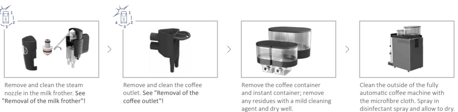
Remove and clean the steam nozzle in the milk frother. See "Removal of the milk frother"!
