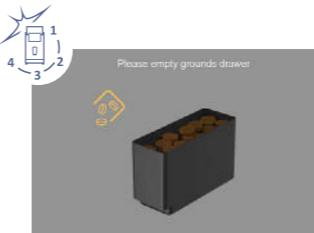
Remove, empty, clean and reinsert the grounds container. After that, press the arrow key to go to the next step.
