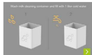
Rinse the cleaning container and fill it with 1 litre of cold water. Then hang the milk aspirator into the cleaning container.
